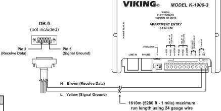
If the RS-232 input of a PC, printer, etc. is capable of receiving TTL level RS-232 signals, then the **LOG BUS** can be wired directly into the RS-232 "Receive Data" and "Signal Ground" pins to receive ASCII data. Windows "Hyper-Terminal" can be used to receive the data on a PC (use the settings in the chart to the left) or visit www.vikingelectronics.com to download free ENTRY LOGGER software (see **Operation** section **E**, "Entry Logger Software").
